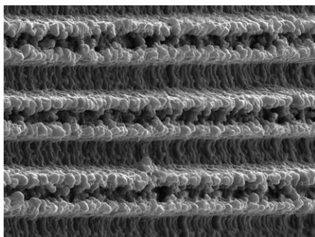
Fig. 1. Laser-microtextured surface (original magnification  $\times 4000$ ).
